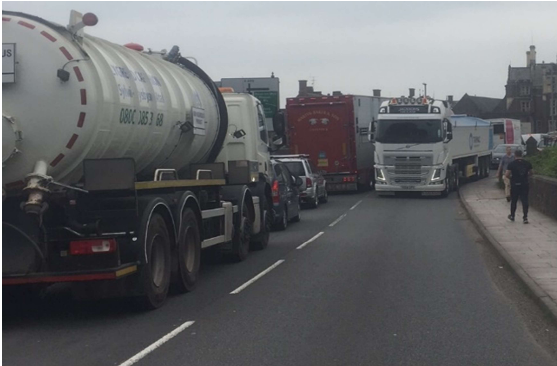
Plate 9 – Multiple HGV Vehicles on the Wye Bridge which has substandard carriageway widths, particularly in this area, where the change of direction causes Heavy Goods Vehicles to drive on the pavement to avoid other Heavy Goods Vehicles in the opposite carriageway.
